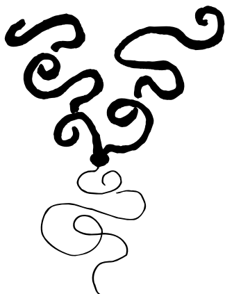
Figure 1. I 2 S graft block copolymer architecture. The dark lines represent PI blocks and the light line represents the PS graft block.
